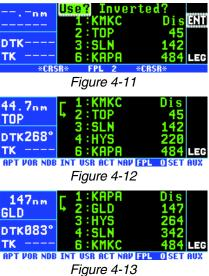
4. The selected flight plan is now displayed as FPL 0, the active flight plan. Any changes made to FPL 0 will not affect how this flight plan is stored as the numbered flight plan.
